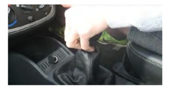
Step 5: Screw on or press the knob onto the lever
